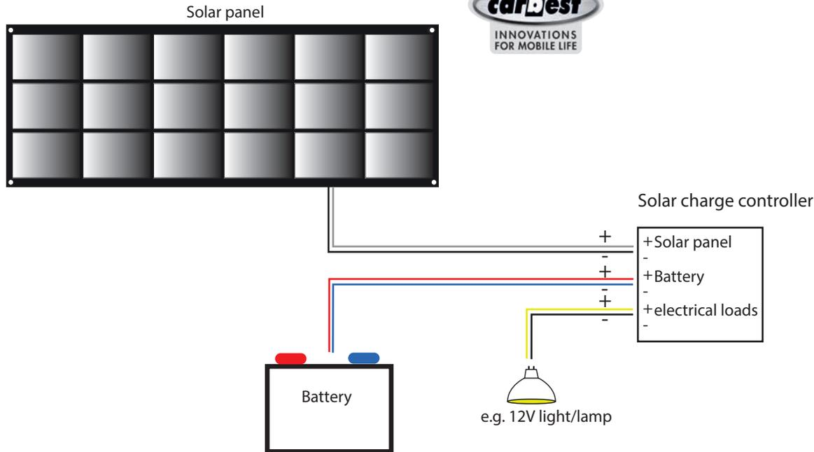
It is recommended to install a solar charge controller between solar panel and car battery in order to avoid an overload / damage of the battery.
