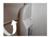
Remove the two screw covers and unscrew the fastening screws beneath. Assembly of the new part is performed in reverse disassembly sequence.
