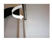
The blind panel must be disassembled as described under **Replacement of blind panel**. Finally, the fastening screws of the guide rails are unscrewed with a Phillips screwdriver. Assemble new parts in reverse disassembly order.
