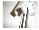
In order to replace the inner cover, the lock plate cover first has to be disassembled as described under 1.7 Replacement of lock plate cover. Then the inner cover (elastic) can be pulled out of the slot. The assembly of the new part is performed in reverse disassembly sequence.
