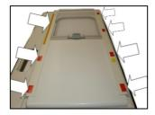
The blind panel should be additionally fixed with double-sided tape at the positions shown in the image to the left. These must be released during disassembly. When assembling the new part, replace the old tape with new tape.
