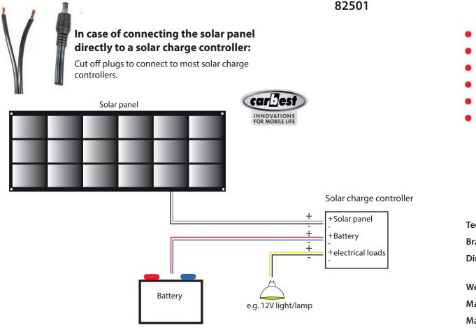
It is recommended to install a solar charge controller between solar panel and car battery in order to avoid an overload / damage of the battery.
