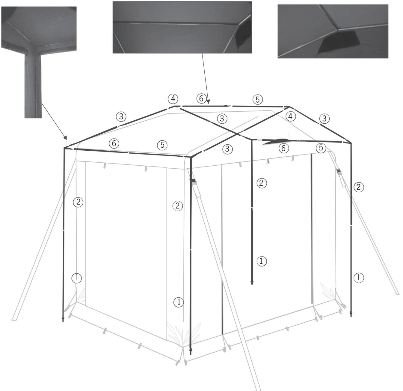
1. a) Assemble the poles like the above drawing, except the leg pole 1
