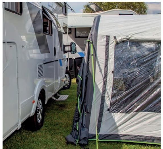
Quick and easy separation and connection of the vehicle thanks to piping with zip fastener
