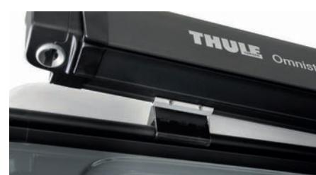
The awning is attached to the REIMO Multirail with the adapters ordered for it. The awning can be disassembled. Only the lower adapter part remains on the vehicle, which lies on the roof.
